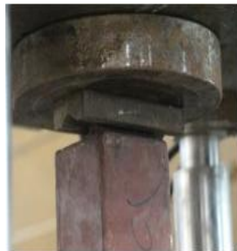
Figure 2. Capping Provided on the Top of Rod during Eccentric Loading
