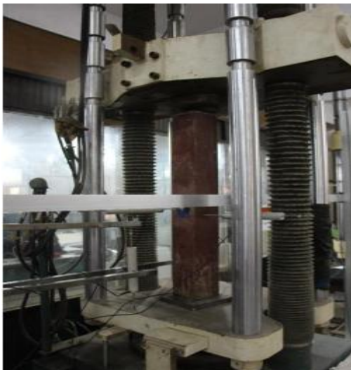
Figure 2. Capping Provided on the Top of Rod during Eccentric Loading
